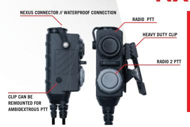
Code Red NX PTT's are a constructed military grade design, not a plastic consumer grade device. The metal alligator clip affixes to uniform/clothing. Both NX PTTs have a Molle clip that can be reversed to be used on left or right side of vest. The NX PTT connection to the headset is waterproof, with a rating of IP67. Can handle watery terrain.
