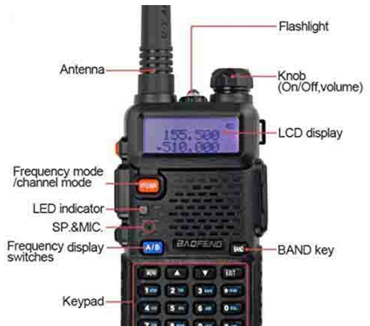
Figure 1: Baofeng UV-5R Diagram (Baofeng Tech)
